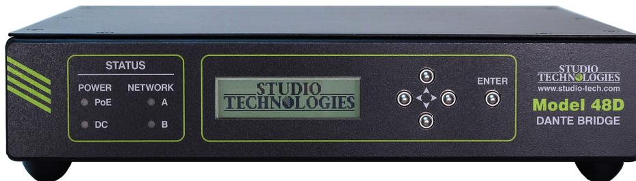
Figure 1. Model 48D “throw-down” front view
