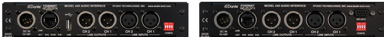
Figure 9. Back view of “original” Model 44D unit with serial numbers 00151-00250 (left) and “updated” Model 44D unit with serial numbers 01151-later (right)
