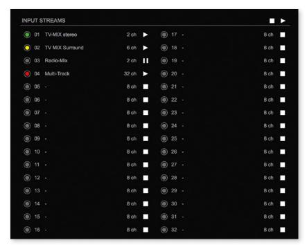
The module can subscribe up to 32 streams. The overview displays the basic information of each stream. The input stream name can be set manually (discovery protocol: manually, see p 54) overriding the SDP's stream name information.
