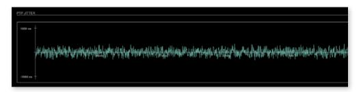
Graphical display of measured PTP jitter.
