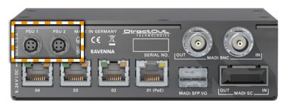
This device may operate with only one power supply. To provide power supply redundancy, it is recommended to connect both PSU 1 and PSU 2 to independent power supplies with separate fuses.
