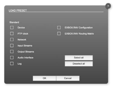
The device configuration can be stored to a single file (.rps).
