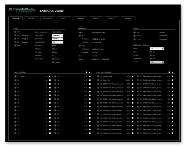
The size of the window and the zoom level can be varied. The page is organized in tabs, pulldown menus or hyperlinks offer access to the values of a parameter. Some values use an input field (e.g. IP address).
