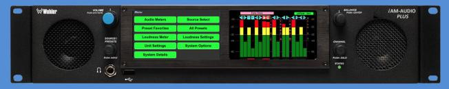
16 channel, dual screen, 3G-SDI & Analog Audio Monitor with optional 2022-7 support, plus options to license additional input signals.
