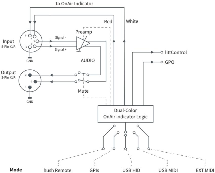
The block diagram above shows the functional structure of the hush+ device. In contrast to hush, hush+ offers you control options for your microphone signal. hush+ comes with a high-quality microphone preamp. It offers you various options optimizing and controlling your mic signal, e.g. a mute function. [See page 31.](#)
