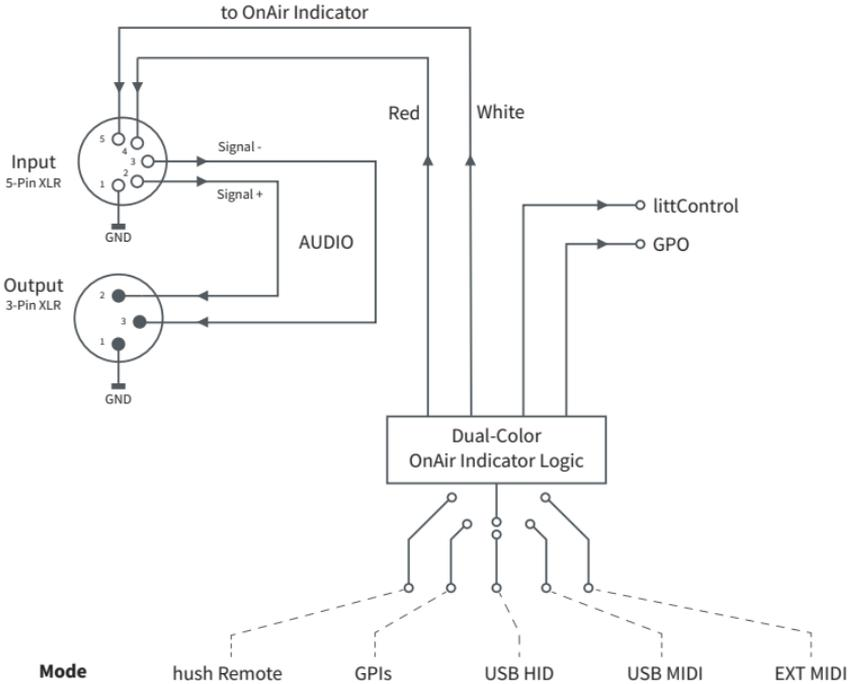
The block diagram above shows you the functional structure of the model hush. Please note that your microphone signal is passed through completely unaffected when using hush. A mute function, for example, is not provided in this variant.
