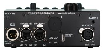
also be used "point-to-point" or interfaced with Dante-compatible matrix intercom systems. The Model 348 includes two Neutrik etherCON RJ45 connectors which allow interfacing with single or redundant Gigabit Ethernet networks. The primary network connection can provide power to the unit using a port on a Power-over-Ethernet (PoE) network switch. It can also be powered using a 12 Volt DC source that is connected using a broadcast-standard 4-pin XLR connector.
