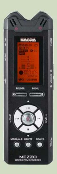
Designed for radio journalist applications, and other hand-held recording opportunities the Nagra MEZZO offers instant start-up, one button recording, automatic level control, internal loudspeaker and a low cut filter. All machine settings are programmed through the comprehensive menu system, where many features of the recorder can be adapted according to the users requirements.
