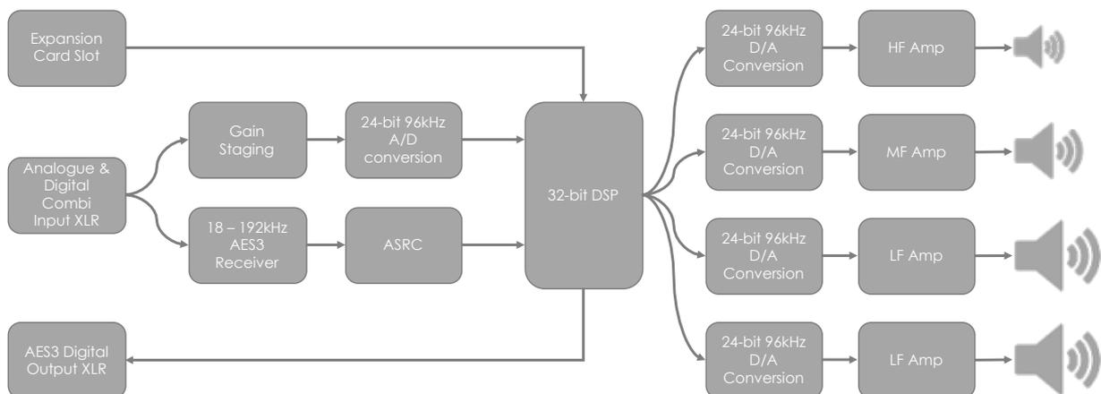
\* The diagram shows 4 channels of amplification, as used in the PMC6-2 and PMC8-2 models.
