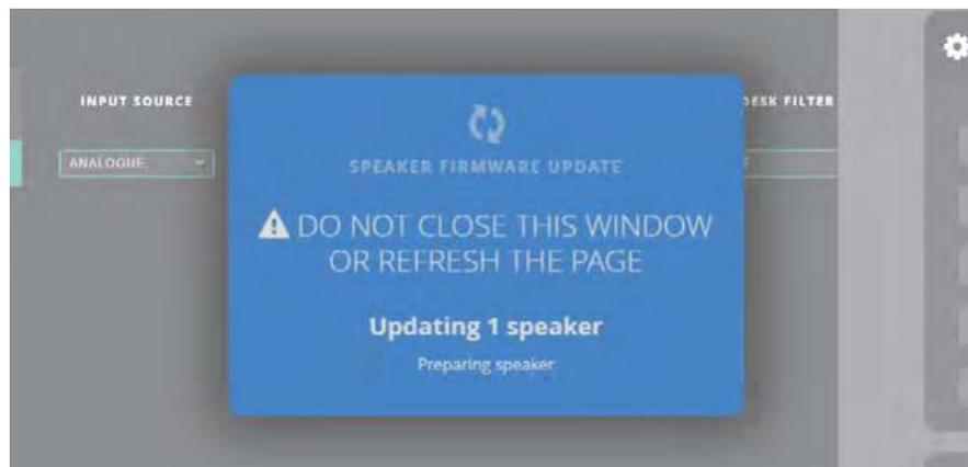
During the firmware update process the speaker's illuminated logo will flash white/blue or white/green. Once the update is complete the speaker will be re-booted and the web-interface will refresh. This process can take up to 60 seconds, and during this time the SoundAlign interface must not be refreshed, or the speaker power cycled or disconnected from the network.
