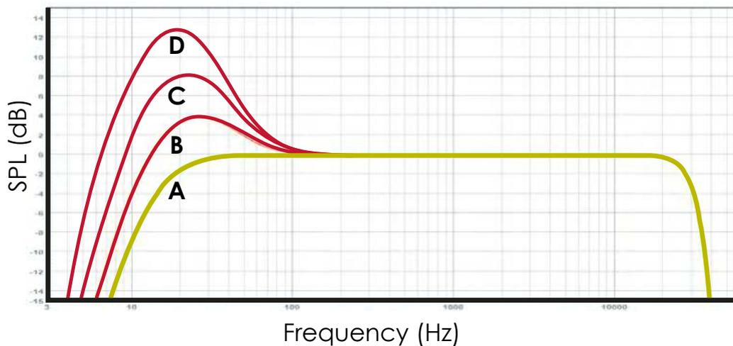
**A:** Free Space is the flat reference setting and no filters are applied. This mode is appropriate if the monitor speaker is placed more than 0.5m (20") away from all walls /ceiling /floor.
