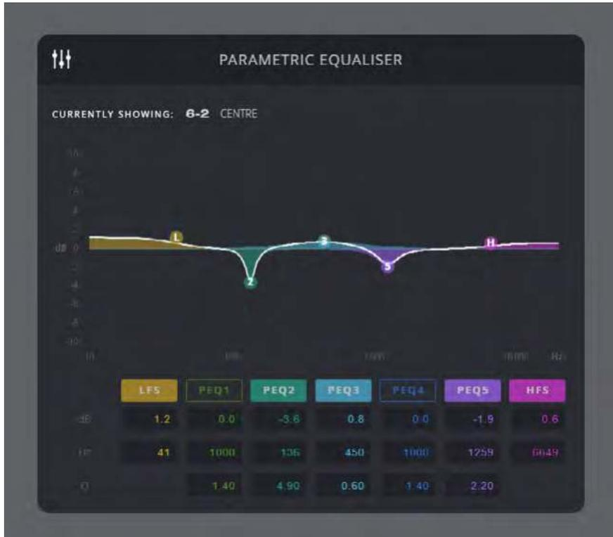
Each EQ band has text entry boxes for each parameter and a coloured On/Off button. The EQ graph can also be clicked and dragged with a mouse, and the mouse scroll wheel adjusts the Q-factor. Altered EQ settings are applied by the DSP only when the mouse button is released.
