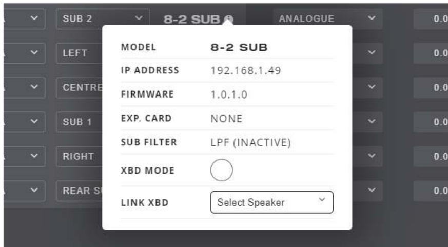
Once the link is formed and the two speakers are merged in the interface, the Model Info box will show information for both speakers. From this extended Info box you can select the input source of the subwoofer cabinet independently of the full-range cabinet, and have the option to unlink the two speakers.
