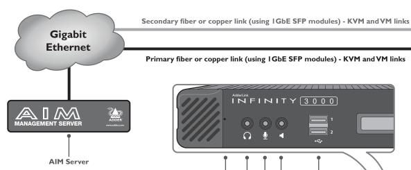
Primary fiber or copper link (using IGbE SFP modules) - KVM and VM links
