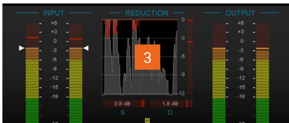
This scrolling history shows input level in grey, and the gain reduction applied in red. This visualisation can be useful to see how much gain is being applied over time, which can be difficult to assess using standard reduction metering. The effect of the look ahead and release controls can also be examined.
