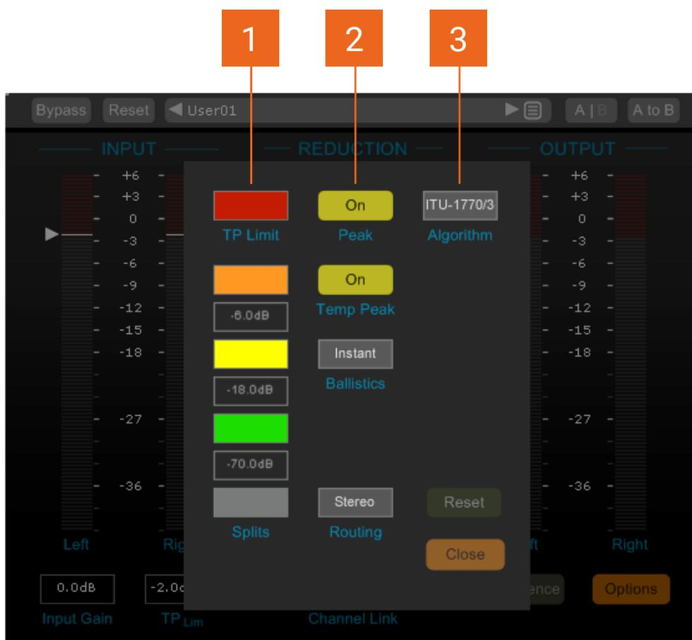
**1 Splits.** This section allows the level meters to be split into colour banding to facilitate the rapid assessment of whether readings are falling within desired ranges or not. The split values determine the position of the colour boundaries. Click-drag up and down to change the value or double click to enter a value directly. To change the colours of the sections, click the swatch to open up the colour picker window.
