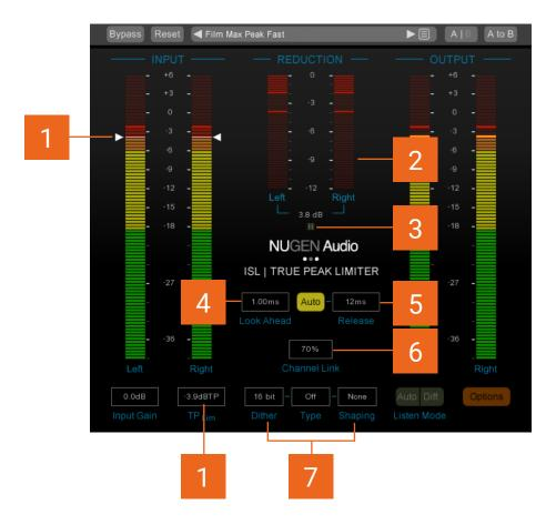
1 TP<sub>Lim</sub>. This parameter sets the True-Peak limit (in dBTP) for the audio signal. Click and drag the mouse up or down to adjust the value. It is also possible to double click and enter a target value directly. This parameter alone will ensure compliance with the TP requirements of current loudness standards.
