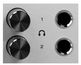
Headphone outputs H1 - H2 with gain adjustment knobs
