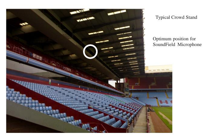
The main wide-shot camera position for any event should be used as the reference position for the SoundField, although this camera position may sometimes not be placed where the main crowd reactions occur. If the microphone has good free space around it, then the aural image will be impressive.
