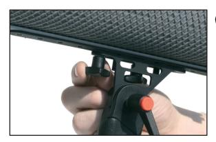
3 Loosen the two black plastic bolts situated on the Pistol Grip under the Windshield.
