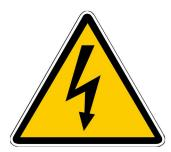
The lightening flash with arrow head symbol within an equilateral triangle is intended to alert the user to the presence of dangerous voltages and energy levels within the product's enclosure that may be of sufficient magnitude to constitute a risk of electric shock or injury.
