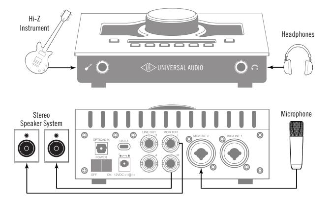
Typical Apollo Twin X USB audio connections. In this example, the mic is connected to channel 2, so the mic and the instrument (which connects to channel 1) can be used at the same time.
