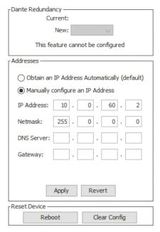
Fig 9: Dante Controller - Network Config in Device View
