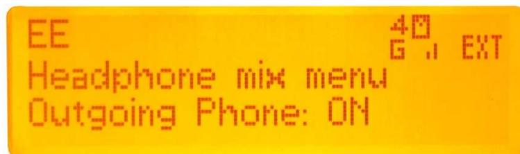
The first setting within the Headphone mix menu is '*Outgoing Phone*' this option allows you to route what you are sending the outgoing phone (i.e. the output of the 2 audio input channels) to your headphones for monitoring. The options for this are 'ON' or 'OFF' to select between the 2 options use the navigation left and right arrows and once the desired option is selected press ENTER to set.
