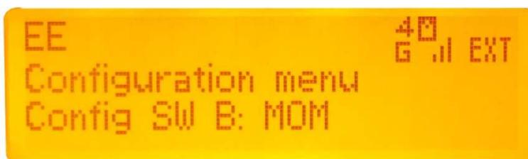
There are 4 options for B Switch Configuration which change how the front panel push switch that turns audio channel B on/ off to the output operate.
