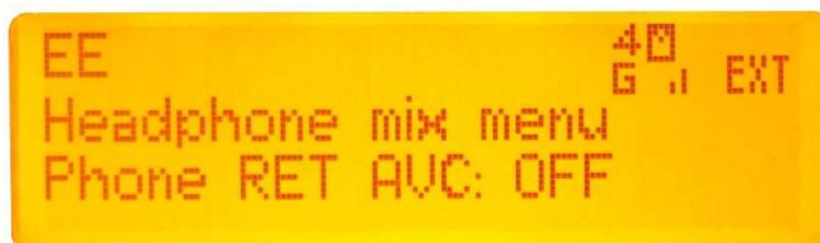
The second setting of the Headphone mix menu is '*RET AVC:*' this option turns on/ off the 'Automatic Volume Control' of the 'Return' audio circuit. This is the audio that is being received by the phone and this option does NOT turn the return audio on/ off but it turns the audio circuit on or off that can automatically adjust the return audio volume for you and increase it if it is too low and turn it down if it is too high.
