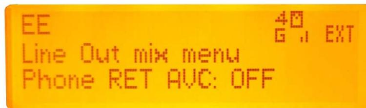
The second setting of the Line out mix menu is '*RET AVC:*' this option turns on/ off the 'Automatic Volume Control' of the 'Return' audio circuit. This is the audio that is being received by the phone and this option does NOT turn the return audio on/ off but it turns the audio circuit on or off that can automatically adjust the return audio volume for you and increase it if it is too low and turn it down if it is too high.
