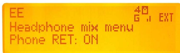
The last option in the Headphone mix menu is '*Phone RET:*' This allows the option of routing the Return audio to the Phone ON or OFF to the headphone mix.
