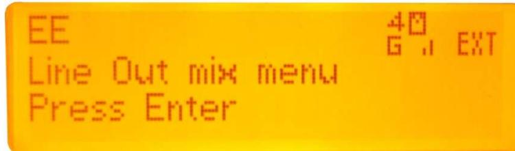
There are 3 settings within the Line out mix menu which allow 2 sources to be routed to the balanced Line output XLR on the side of the Expedition. To access these settings press ENTER.
