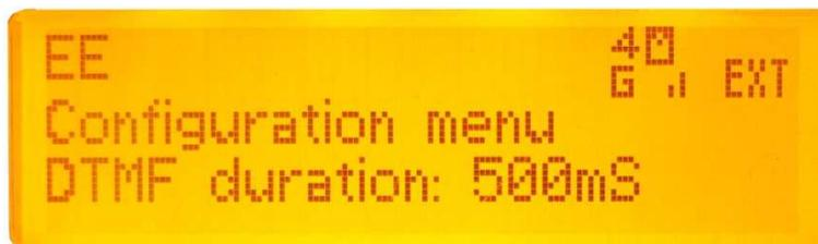
Once a call is in progress pressing one of the keypad buttons (0 – 9, \* and #) will send the appropriate equivalent 'DTMF' tone to the phones output. The length of this DTMF tone can be changed in this menu between 500mS, 1000mS and 2000mS. To change the current setting use the navigation left/ right arrows to select the desired duration and press ENTER to save.
