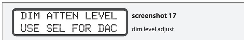
3. To increase the dim dB value, rotate the main level encoder in a counter-clockwise direction. As you do this, you'll see the dim settings change in 5dB increments. Rotate the encoder in a clockwise direction to reduce the dim level.
