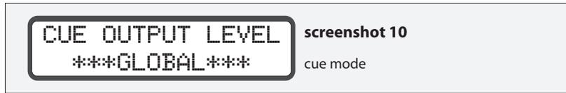
4. Rotate the 'main level/edit' rotary encoder in a clockwise direction to increase the value. Rotate the encoder in a counter-clockwise motion to decrease the value. The individual Left and Right levels can be trimmed as well by pressing the "Left" or "Right" buttons in the solo/mute button row. The trim range for each channel is +/-10dB (screenshot 11).
