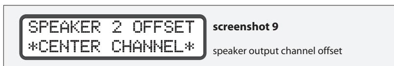
3. Now press any of the channel solo/mute switches belonging to the individual speaker channel you want to modify. Its switch LED will begin to flash. You can select another channel to edit at any time simply by pressing its associated switch.
