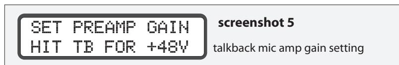
3. To increase the mic amp gain, rotate the main level encoder in a clockwise direction. As you do this, you'll see the gain settings change. Preamp gain is adjustable from +30 to +70dB in 3dB steps. Rotate the encoder in a counter-
