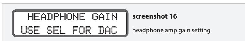
4. Rotate the 'main level/edit' rotary encoder in a clockwise direction to increase the amplifier gain. Rotate the encoder in a counter-clockwise motion to decrease the value. The output will change in real-time (gain settings of 0dB, 10dB and 20dB are available).
