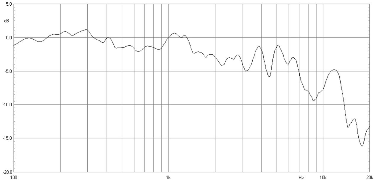
Displayed range from 100 Hz up due to measurement room size limitations.
