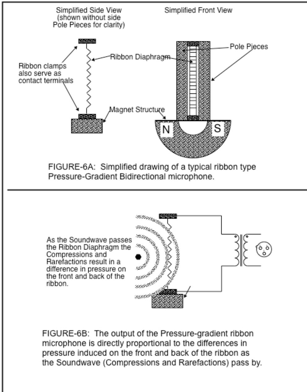
Because these were dipoles, if a soundwave approached the diaphragm directly from either the front or back, the ribbon would move equally. The only difference was the absolute polarity of the electrical output: sounds arriving from the back produce polarity opposite to those arriving from the front. (ref. Figure 7A and 7B)
