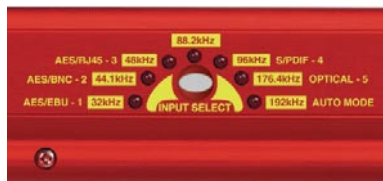
Fig 1-2: RB-DDA22 Front Panel Controls
