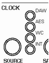
The 'CLOCK SOURCE' display indicates which input is acting as a clock reference for the ADC16. The indicators are as follows:
