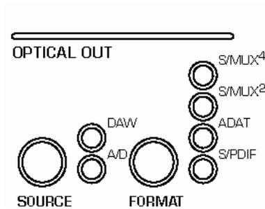
The optical output can provide either AES/EBU or ADAT format. The AES/EBU mode works with most S/PDIF optical inputs.
