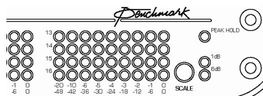
The 'SCALE' button selects the scale and peak-hold mode of the 9-segment LED Meter Display.
