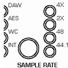
The 'SAMPLE RATE' button sets the sample rate when the ADC16 is in the 'INT' clock-source mode. This button is only active when the 'INT' LED is on.
