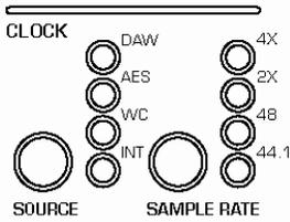
The 'CLOCK' control interface consists of a 'CLOCK SOURCE' button, a 'Sample Rate' button. Each button has a corresponding LED display.
