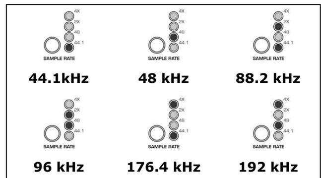
The 'SAMPLE RATE' LED display always indicates the sample rate at which the ADC16 is operating.
