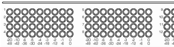
The ADC16 is equipped with a multi-function 9-segment LED meter. The 'SCALE' button selects either a 6 dB step or 1 dB step scale and controls the peak-hold function. Metering is fully digital and post-conversion for absolute accuracy. The units are dBFS (dB relative to the maximum possible digital signal).
