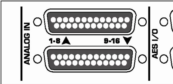
The balanced "ANALOG IN" line-level inputs follow the Tascam Analog DB-25 standard. Cables are available from many sources.
