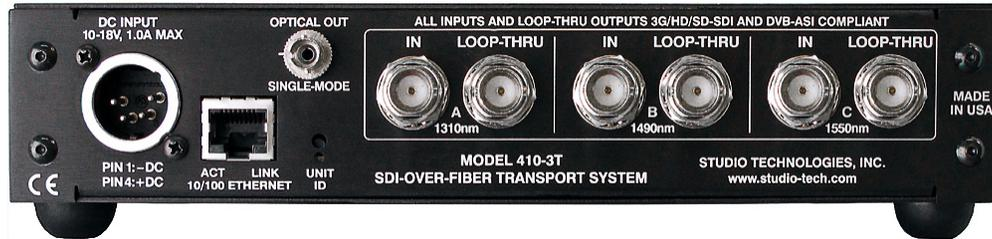
The Model 410-3T provides electrical-to-optical (E2O) conversion of 3 SD/HD/3G-SDI inputs to 1 single-mode optical output. BNC input and loop through connectors (6 total); ST optical output connector (1 total).
