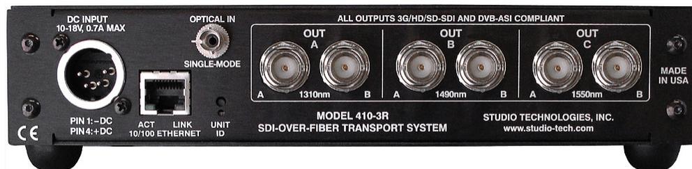
The Model 410-3R provides optical-to-electrical (O2E) conversion of 1 single-mode optical input to 3 pairs of SD/HD/3G-SDI outputs. ST optical input connector (1 total); BNC SDI output connectors (6 total).
