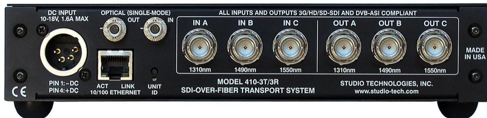
The Model 410-3T/3R provides both electrical-to-optical (E2O) conversion (3 SD/HD/3G-SDI inputs to 1 single-mode optical output) and optical-to-electrical (O2E) conversion (1 single-mode optical input to 3 SD/HD/3G-SDI outputs). BNC SDI input and output connectors (6 total); ST optical output and input connectors (2 total).
