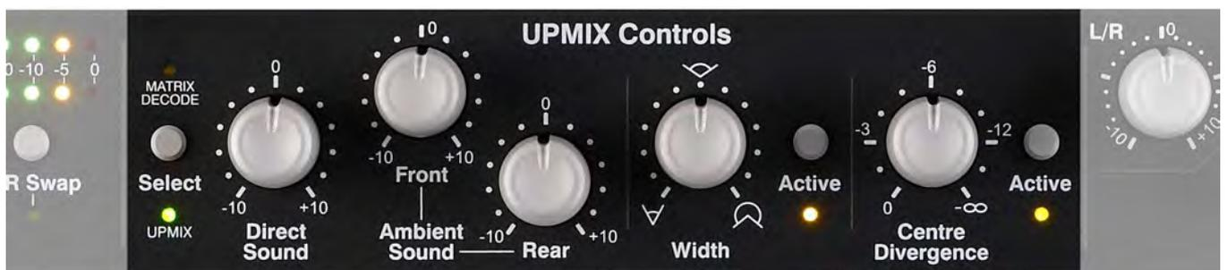
There are three controls central to the UPM-1's operation: Front Direct Sound, Front Ambient Sound and Rear Ambient Sound. By adjusting these three controls the user can create a desired balance between direct and ambient sound within the 5.1 surround. Two further controls, Width and Centre Divergence, provide the opportunity for further fine adjustment to imaging and centre channel content. Output level controls are provided for the Front, Rear, Centre and LFE channels.
