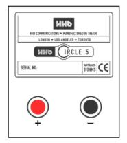
area, since this will reduce the electrical resistance. If the cable is too thin, the resistance rises and heating may occur. Also, try to keep the length of cable from the loudspeaker to the amplifier short to keep the induced noise as low as possible. Where possible, use the same length of cable for each speaker.
